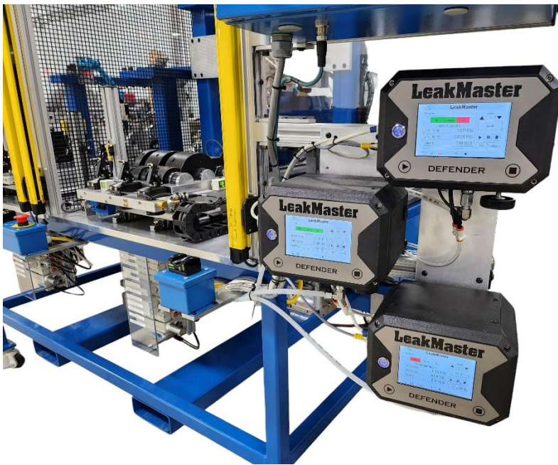
Custom Automated turnkey leak test system with multiple Defender leak test instruments.
